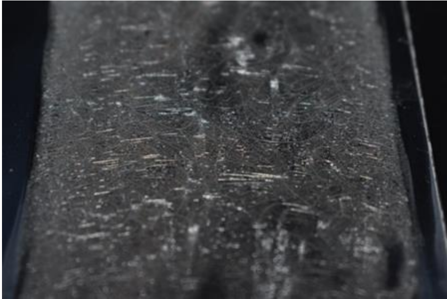
Surface Defects on a 150 \mu\text{m} Film of Pure SETAQUA® 6462
