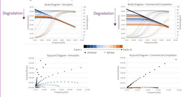
As seen in the graphs above, the coatings degrade with each cycle. The sample based on the commercial competitor shows a very low corrosion resistance, and fails after only two cycles. The sample based on Amorphic degrades more slowly with each cycle and shows higher impedance values (higher barrier) than the commercial competitor. After the 12 cycles, the Amorphic-based coating doesn't show any damage, which confirms its superior anti-corrosion performance.
