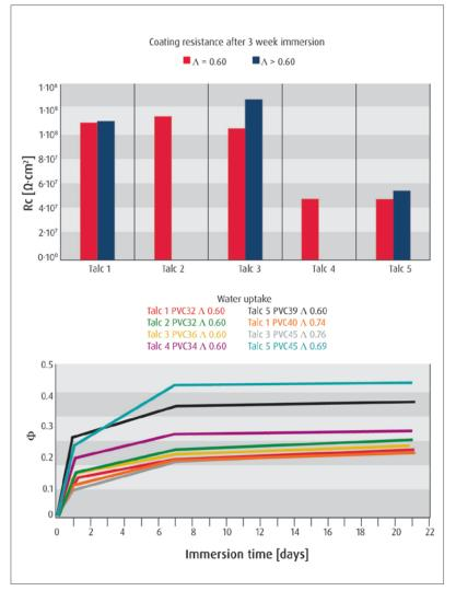
Figure 2: Coating resistance (Rc) and water uptake ( $\phi$ ) evaluation
