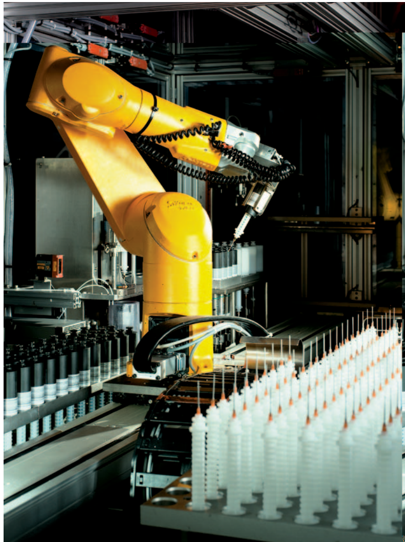
Paint maker Wörwag has been operating a fully automated high-throughput plant in its combinatorial laboratory since 2006
